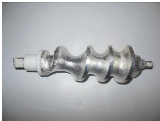
**Fig.2-2 Vite elicoidale**
